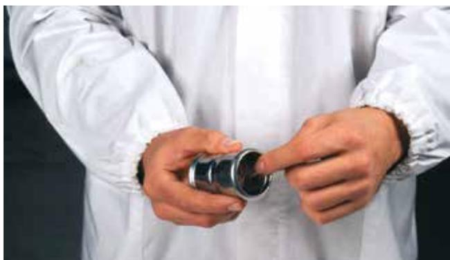
**Figura 30** - Controllo O-ring
