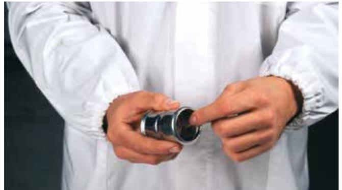
**Figura 25** - Controllo O-ring
