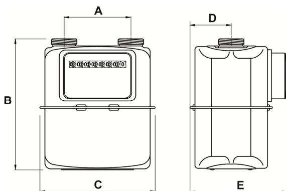
**PER CONVERTIRE I METRI CUBI DI GPL IN FASE GASSOSA MISURATI DAL CONTATORE IN LITRI DI GPL IN FASE LIQUIDA, OCCORRE MOLTIPLICARE PER 4,166 IL NUMERO LETTO SUL QUADRANTE.**
