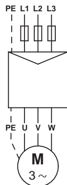
Fig. 14 Grundfos motors, direct-on-line starting
